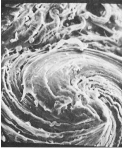
Fig. 8. SEM fractography ( \times 100 ) of the core of a solid specimen tested at 5 kbar.
