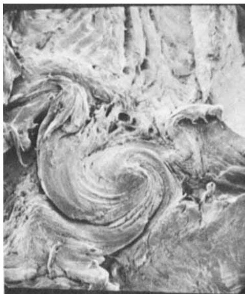
Fig. 7. SEM fractography ( \times 27 ) of the core of a solid PP specimen tested at 5 kbar.
