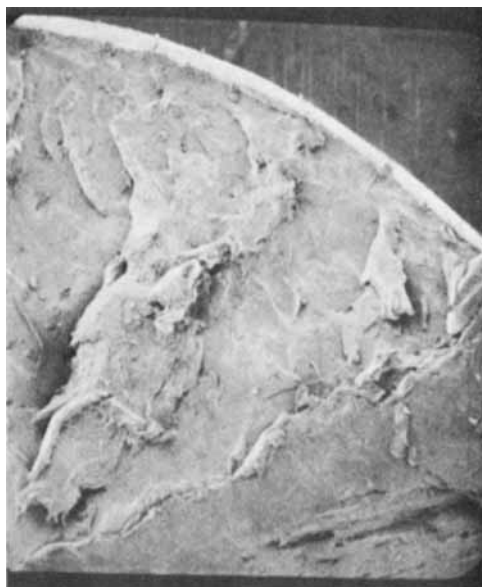
Fig. 6. SEM fractography ( \times 27 ) of the edge of a solid PP specimen tested at 5 kbar.
